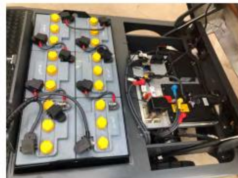
ST3000-AC tow tug complete with 6 x 250AH heavy duty batteries
